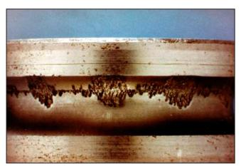
Figure C1. The bearing damage shown here corresponds to the spacing of the rolling elements. It started as non-rotating vibration during shipping or storage.
